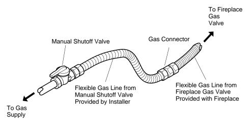
Figure 24 - Attaching Flexible Gas Lines Together
